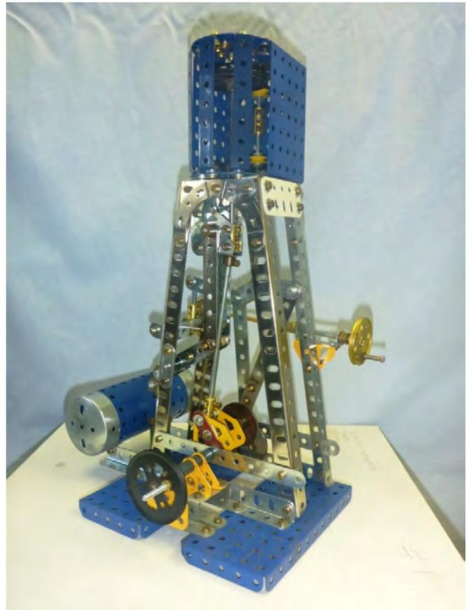
The representation in this model of the main elements in a single-cylinder marine steam engines is quite good. The elements include a reversible Stephenson's Link, a thrust block, condenser and bilge pump driven by links to the crosshead slide.
