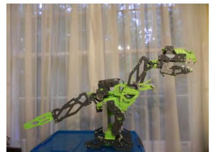
The hip section has a sealed motor and gears powered by four C batteries with a control unit fixed on top. The control unit has a light sensor, microphone and speaker with buttons for directional movements, attack, room guard, question and answer, recording and playback. The model is not remote-controlled.
